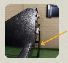
**4.** Move the bracket inwards on the load bar until the flat mounting surface of the bracket protrudes over the load bar. (This leaves enough space for the end cap to sit flush with the bracket)
