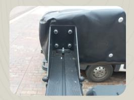
**6.** When the Bracket is secured to the load bar, you can fit the awning.
